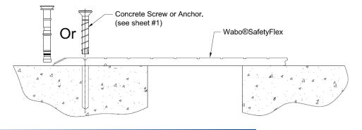
For a wall termination, use a Heavy Duty saw (Worm Gear type recommended) with cutting blade for Steel to cut Wabo®SafetyFlex. Leave about a 1/16<sup>°</sup> gap between Wabo®SafetyFlex and the wall. Fill in the 1/16<sup>°</sup> gap with a bead of silicone sealant (By Others).
